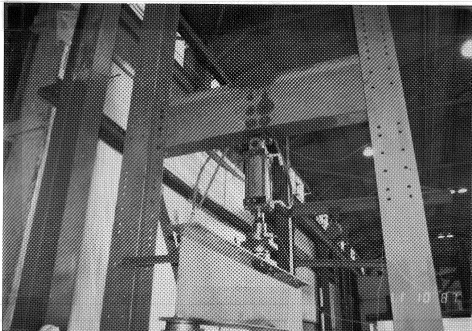
Figure 3.11 Photographs of the Loading Frame
